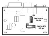
Figure 4: Switch Locator
